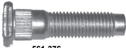
561-376 M12 x 1.5 x 49mm Knurl diameter: 13.9mm
