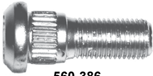
560-386 7/16-20R x 1-5/16" Knurl diameter: .555 (Code: DN)
