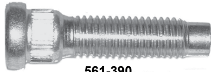
561-390 M12 x 1.75 x 51mm Knurl diameter: 14.73mm
