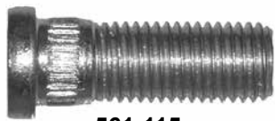
561-115 M12 x 1.5 x 35mm Knurl diameter: 12.7mm
