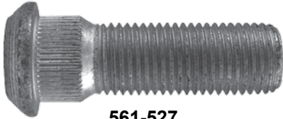
561-527 M14 x 1.5 x 45.5mm Knurl diameter: 16.5mm
