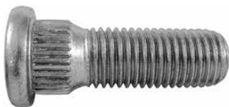
561-114 M12 x 1.5 x 38mm Knurl diameter: 14.35mm (Code C.U.1)
