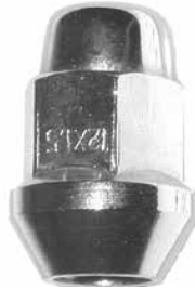
559-077 M12 x 1.5 19mm (3/4") Hex 35mm Height Cone Angle: 60° Acorn Bulge Chrome
