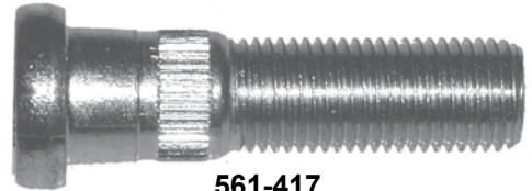
561-417 M14 x 1.5 x 54mm Knurl diameter: 15.7mm (Code DK)
