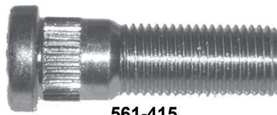
561-415 M14 x 1.5 x 46mm Knurl diameter: 15.8mm (Code DO)
