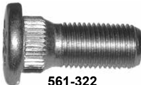
561-322 M12 x 1.25 x 30.2mm Knurl diameter: 14.27mm
