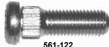
561-122 M12 x 1.5 x 36mm Knurl diameter: 14.3mm (Code T.5.0)
