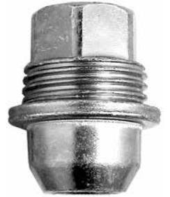
559-151 M12R x 1.5 19mm Hex 34mm Height 60° - Flanged Flat Yellow Zinc
