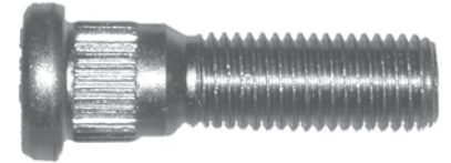
561-312 M12 x 1.5 x 44.4mm Knurl diameter: 14.17mm
