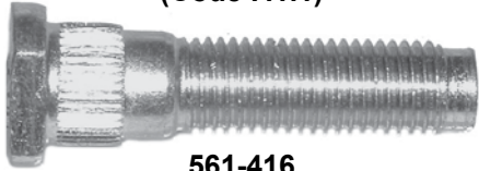
561-416 M12 x 1.5 x 52mm Knurl diameter: 14.8mm
