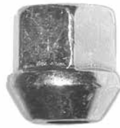
559-163 M12 x 1.5 19mm (3/4") Hex 23mm Height Cone Angle: 60° - Zinc
