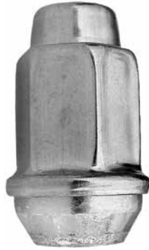
558-094 1/2-20R 3/4" Hex 1-39/64" Height Stainless Steel Capped
