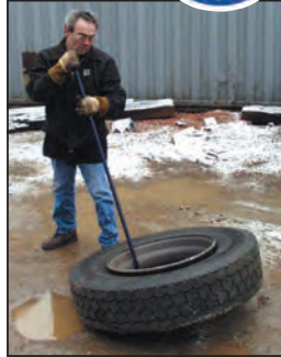
Specially designed forged ends work from either side of the wheel assembly as it lays flat
