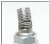
Galvanic corrosion causes TPMS failures.
