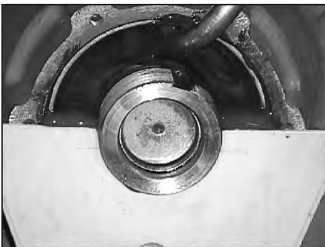
Fig. 5: Semi-Fluid Grease Top Off Procedure
