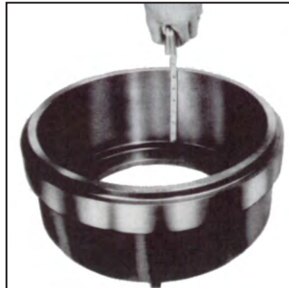
Width of braking surface
