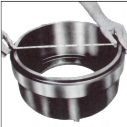
Diameter brake surface (allow for drum wear)
