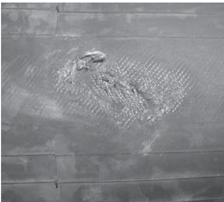
Abrasion of the rubber bellow - is caused by an object constantly rubbing on it, ultimately creating a hole.
