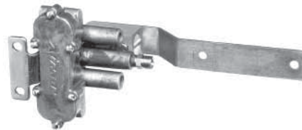
HEIGHT CONTROL VALVE
