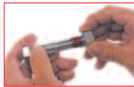
4. Assemble parts and tighten to recommended torque.
