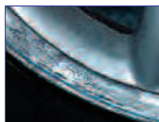
Curbside Rash & Scuffs
